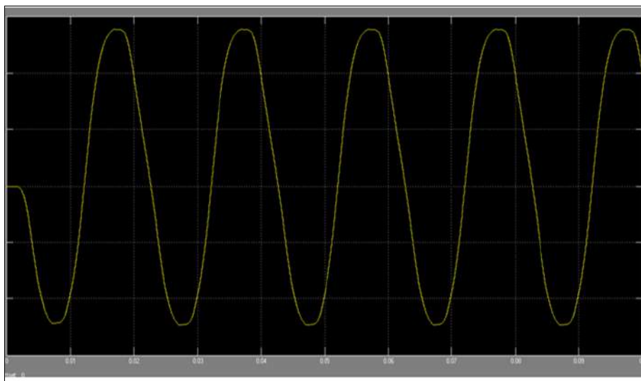
Fig 7: Output voltage waveforms of a filtered single-phase seven-level asymmetric CHB MLI
