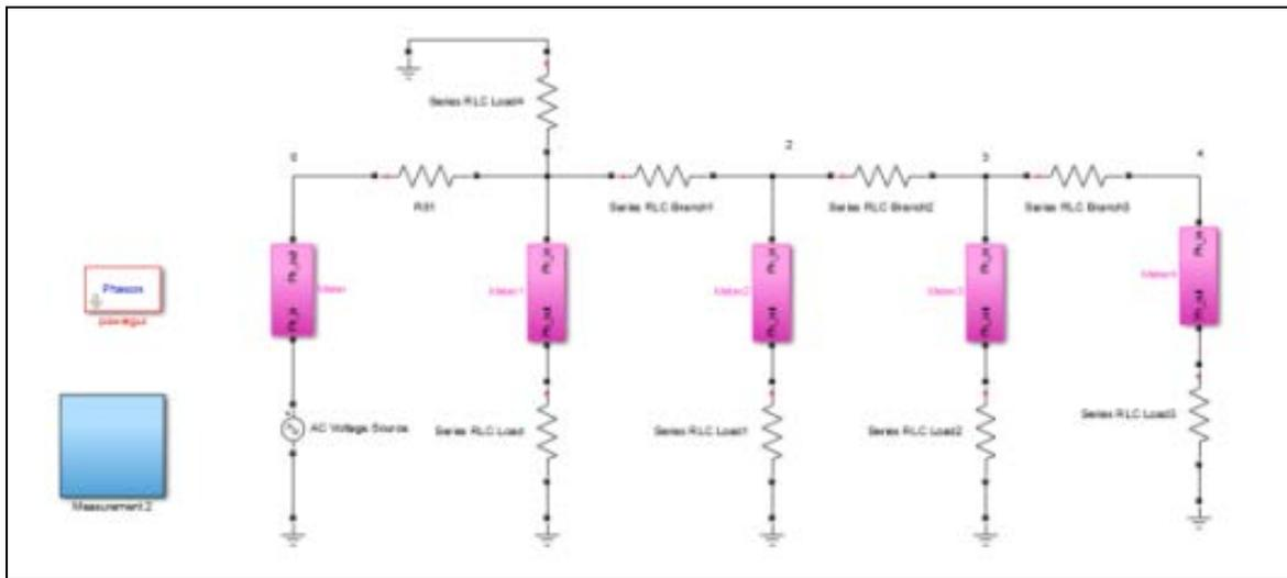
**Fig 5:** Simulink Model of the Distribution System
