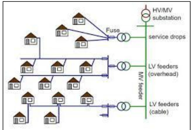
Fig 3: Radial Distribution System
