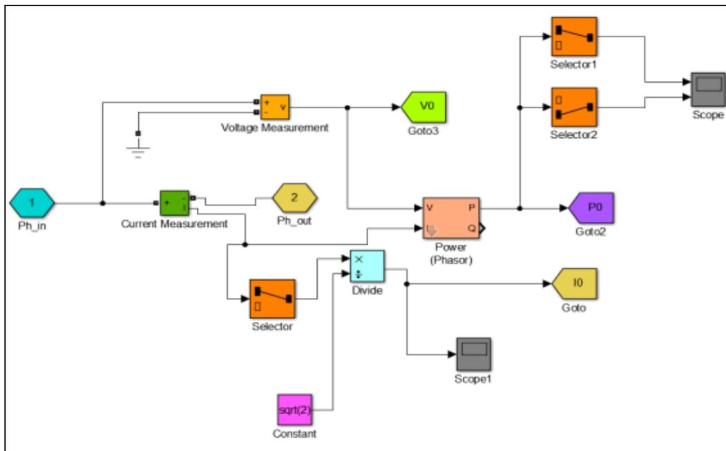
**Fig 6:** Simulation Sub-System of the Smart Meter
